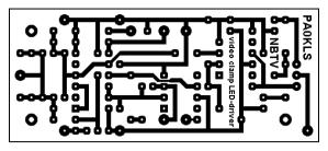
are two wire links to be placed, one of them under the circuit HEF4053. So first solder the link in place before you place the IC.
