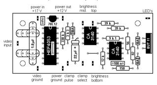
There are several holes to hold the video capacitor of 1.8  $\mu$ F. A rather large colour banded polyester capacitor was used in the prototype. Always use a good quality capacitor, never an electrolytic capacitor in this place. You may use a smaller sized 1  $\mu$ F with 0.82  $\mu$ F in parallel.
