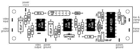
For the first test preset the 1k trimmer pot slightly below its centre position. The complete circuit needs just a few mA of power, so it can be fed from the stabilised 12 volts that is built in the NEON/LED driver. Adjust the contrast input potmeter to get 1.4 volts peak/peak video measured on the video output pin. Then you should have stable line and frame pulses. If this is not the case then adjust the 1k trimmer pot. Photograph on the next page.
