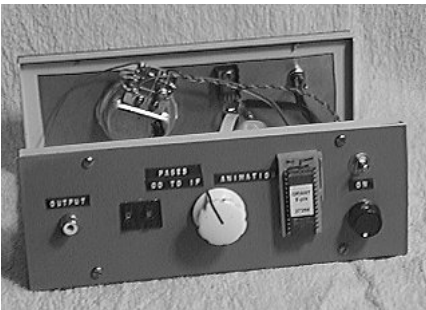
Front panel of the prototype unit. The socket on the PCB is connected to a ZIF socket on the panel by means of ribbon cable.
