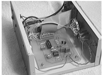
The 2-way switch is a rotary wafer type. The current PCB design is not the same as that which is shown here.
