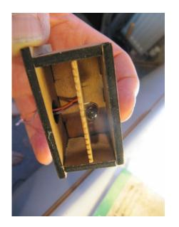
Place the two pieces of stripboard inside the two enclosures as shown here on the left, align the two components then glue the stripboards into position. Feed the two cables through the bottom of the units. Store the two completed units safely.
