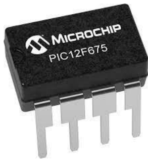
Programmed PIC for Chris Lewis's control board
