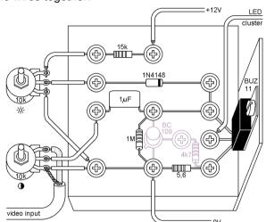
Screw the transistor to a small piece of aluminium sheet so it can get rid of its excessive heat and fix the wires to the lugs of the potentiometers by soldering. The overload protection is shown in grey.
