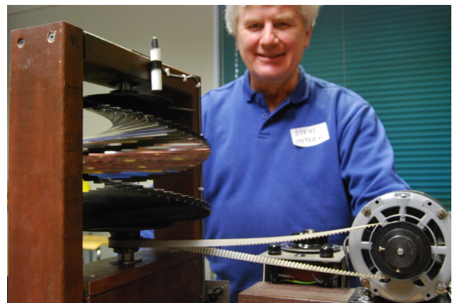
Left: Loughborough Convention, April. Light line-source on tripod. Right: Drive from induction motor. See sync pickoff at top of frame.
