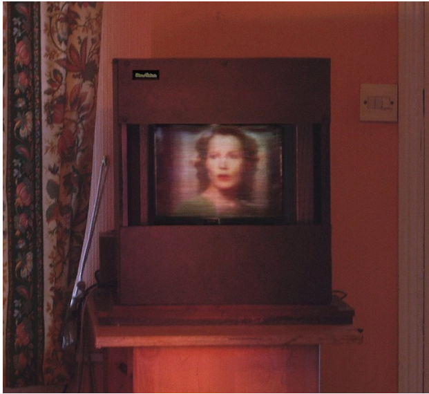
The screw operating at 60-lines. This was shown also at our April Convention. Right, the mirror screw built for 120-lines.
