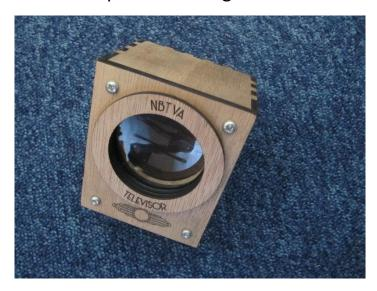
Although a laser-cut support frame has been designed for the televisor the 50mm lens taken from a handheld magnifying glass was deemed too small although we have laser printed assembly and are able to supply design files so cutting can be carried out locally. We recommend you experiment with lenses you have available.
